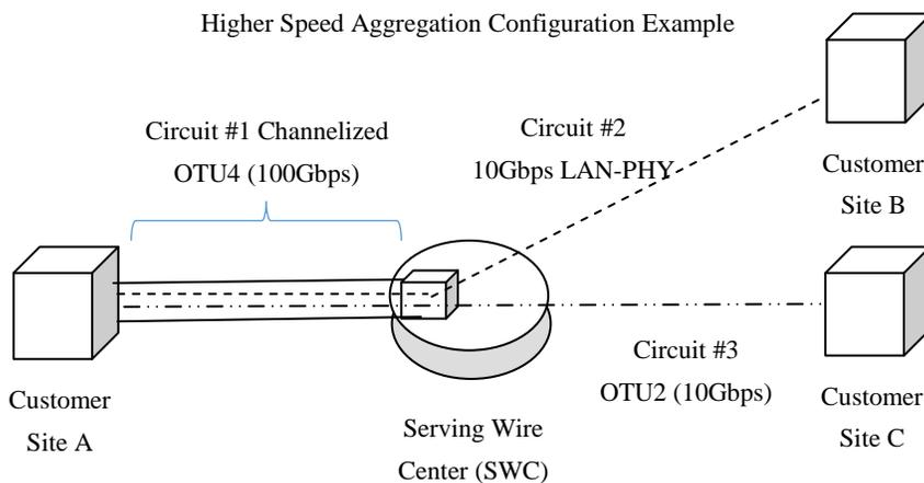
In the example of a higher speed aggregation arrangement depicted in the diagram above, there are three AT&T Dedicated Ethernet circuits, as follows:
